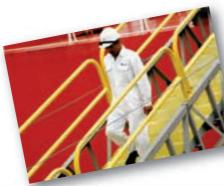
Guardrail Systems: You see this system at work everywhere you see a balcony. This is the rail that must exist above the edge of platforms. This guard rail will keep you from falling off the edge of a platform. The top of this rail must be 42 inches high above the platform.
