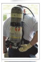
another type of Air-Supplied Respirator. This type of respirator uses a tank of air that you carry with you. A self-contained breathing unit (SCBA) MUST be used if the conditions of the air are not known OR where the air is Immediately Dangerous to Life and Health (IDLH). Different SCBA's may last between 5 minutes to 45 minutes. 5 minute units are only to be used for escape or emergencies.
